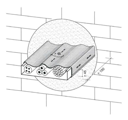
For some fire resistance classifications (see annex D-1 of the ETA) it is necessary to wrap strips of "FBA-WI" of at least 150 mm width on both sides around cables or cable trays.
