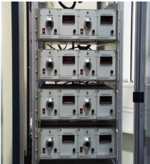
Photo 2 : View of the charging units inside a cabinet.
