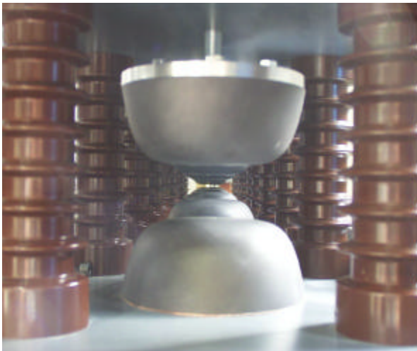
Photo 5 : View of Spark gaps of one bank of 5 units.
